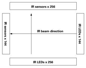
If the conventional scanning method is used, it would be possible achieve resolution of only 256 x 144 as shown above. However, the scan device also performs scanning in the oblique directions and computations for achieving high resolution to match the plasma display monitor pixels (1280 x 768).
